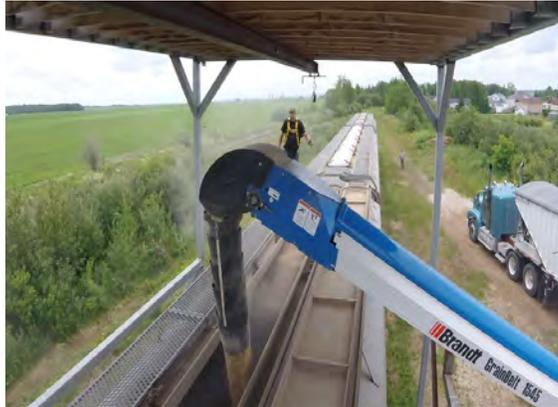
*The farm's loading system to transfer agricultural product from truck to covered hopper railcar on ONTC's spur line.*
